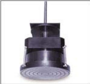
Compression testing can utilize the spherical seating platen to ensure even loading.
