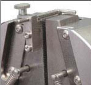
Some grips and fixtures feature specimen stops that allow the specimen to be accurately and repeatably located.
