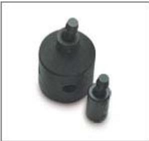
[Flexible or universal couplings](#) can be employed to allow the grip to align itself with a slightly bent specimen. Some types of grips employ two universal couplings, one at the top and one at the bottom.
