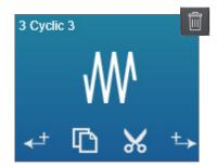
Key step controls - insert, cut, copy, paste and delete - are located within the step, reducing the amount of time putting steps together as compared to a traditional menu or toolbar-driven design
