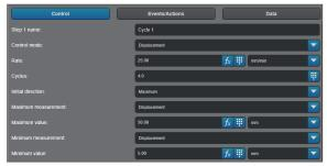
Making the test parameters user-driven variables gives you an easy way to rapidly change test parameters right from the operator screen. The powerful Bluehill® Universal Expression Builder makes this seamless in TestProfiler.
