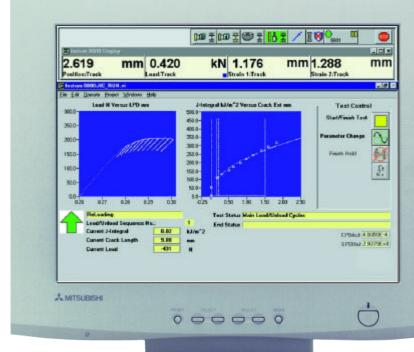
For each sequence, the J-Integral value and the crack length are calculated and stored in an ASCII file. Realtime graphics of load versus load point displacement and J-Integral versus crack extension keep the operator informed of the status of the test. Based on this data, modifications to test parameters can be made as the test is running.
